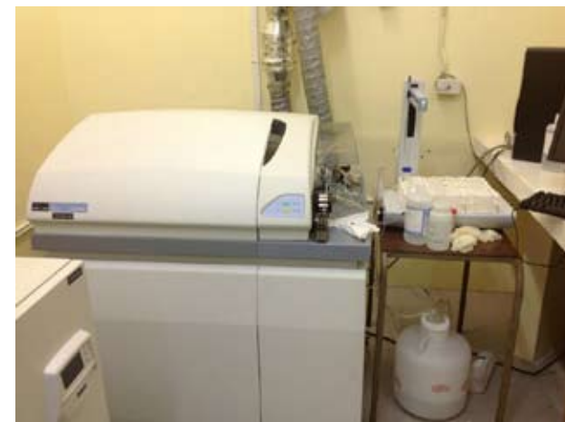
Inductively coupled plasma mass spectrometer (ICP-MS) used to determine very low metal concentrations in a variety of samples.
