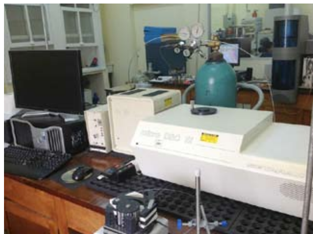
Differential Scanning Calorimeter (DSC) used to measure heat flow in a sample in order to gain information about its structure.
