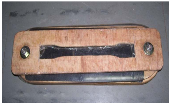
Figure 1. ITR-EC tensile test specimen production rig
